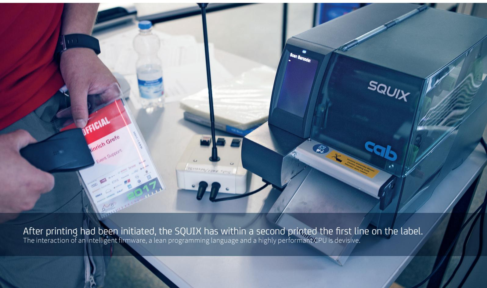
After printing had been initiated, the SQUIX has within a second printed the first line on the label. The interaction of an intelligent firmware, a lean programming language and a highly performant CPU is decisive.
