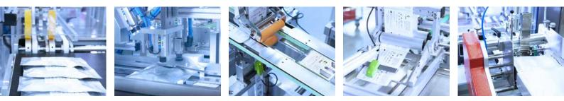
Specified machines are constructed, assembled and initially operated at the Kraus facility in Spaichingen, as well as accepted by the customers prior to delivery. In the operation at hand, Plexiglas replicas of LifePad PCR test cassettes and three-side sealed pouches are fed by friction feeders from preceding processes to a machine combined for labeling and packing.
